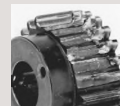
Example of failure due to insufficient bending strength
