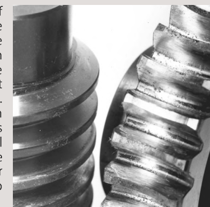
Example of wear due to insufficient surface durability
