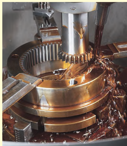
Gear cutting by CNC Gear Shaper
